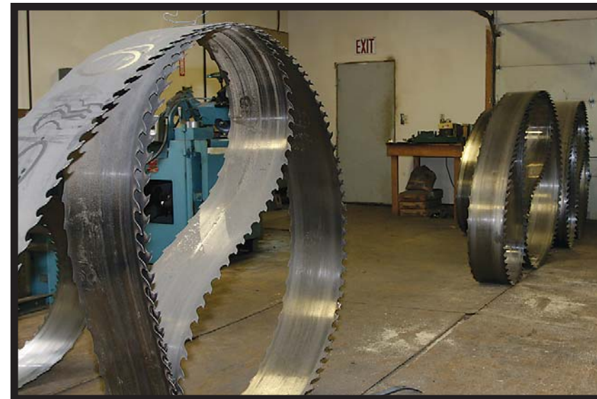
Forty feet long and one foot wide, the giant closed loop saw blades are changed every four hours minimum. Production slows down when they saw particularly hard wood such as hickory or ash.
