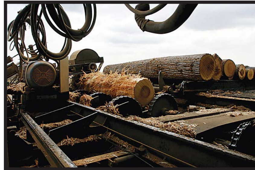
The de-barker does its job and sends the bark to the mulch pile.
