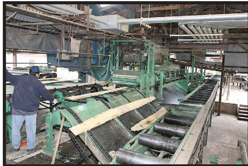
As a worker operates a laser-sighted saw, unused slabs are dumped below to a conveyor belt that will take them to a chipper. The chips eventually will be shipped to a pulp mill to become paper.
