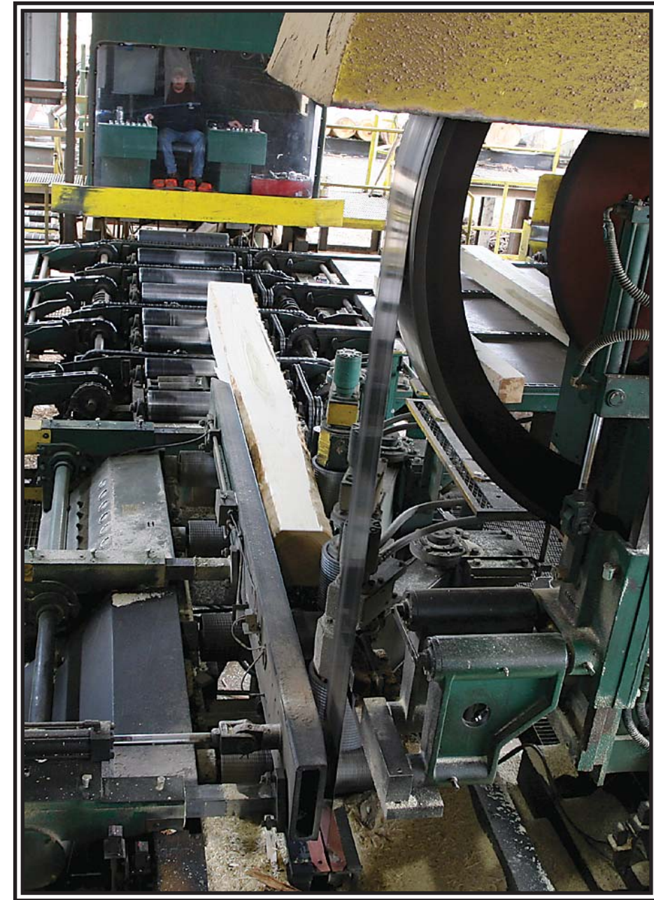
Above, after the head rig turns a round log into a square one, it is shunted to the line bar re-saw in the foreground, which transforms it into planks. Note the saw operator in the booth at the top of the photo. Below, R.S. Coleman Lumber is a family affair. Sandy Coleman works in the sawmill office, Robert buys the timber tracts, and their son Jamie runs the sawmill operation and markets the wood. Note the hardwood mulch pile in the background.
